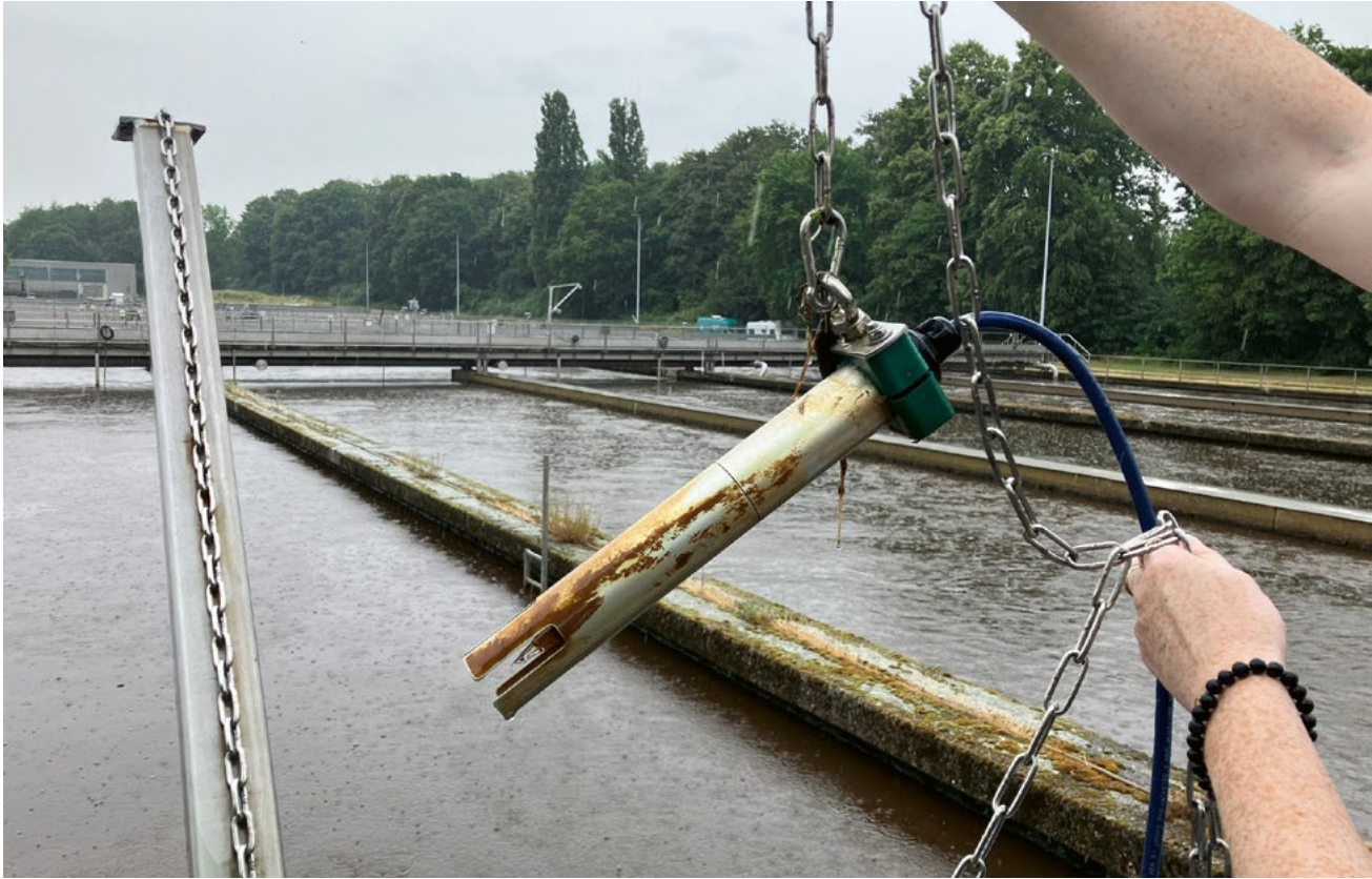
The bioSpectre project by Okeanos GmbH in Bochum aims to measure hard-to-detect wastewater quality parameters almost in real time using innovative sensors.
