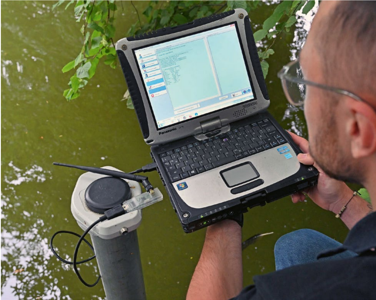
The City of Bochum monitors the quality of its blue-green infrastructure's waterways using sensor technology.
